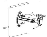
A: Screw of vertical adjust; B: Screw of Horizontal adjust
