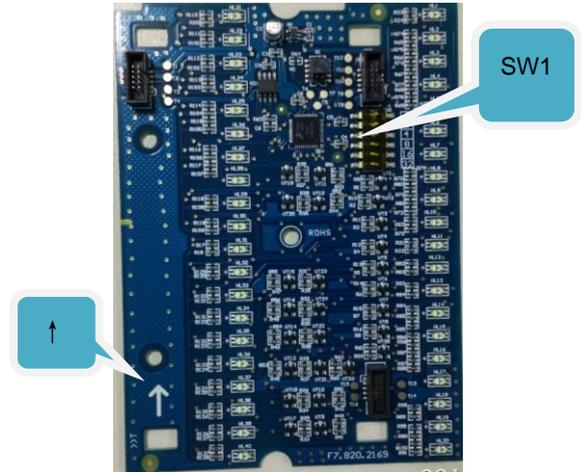
Fig. 2 ZC-400 Zone Display and Control Board
